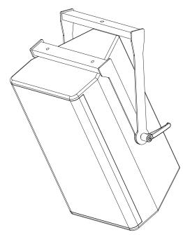
Ensure that both the flat and locking washers are used – the flat washer should be in contact with the cradle. Tighten the bolts to ensure a solid fit. Once the desired angle of the loudspeaker is set, tighten the levers on the cradle to lock the position in place. The points on the top of the flying cradle can be used for permanent installations or to secure a hook clamp.
