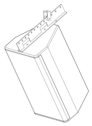
Using the supplied M10 hex head bolts, align the mounting holes in the flying bracket with the mounting points on the top or the bottom of the enclosure. Ensure that both the flat and locking washers are used — the flat washer should be in contact with the cradle. Tighten the bolts to ensure a solid fit. Finally, attach a hook-clamp to the mounting point.
