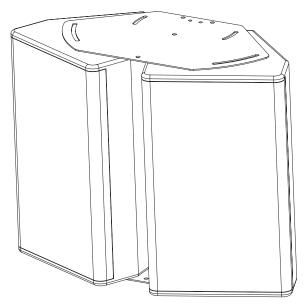
Using the supplied M10 socket head bolts, bolt through the CP-XY12DF1 plate into the enclosures. Ensure that both the flat and spring washers are used — the flat washer should be in contact with the plate. Once the desired angles of the loudspeakers are set, tighten the bolts to lock in place. Then turn the cluster over and repeat the process on the bottom. Use the top points on the XY-122 enclosures as a secondary safety feature.
